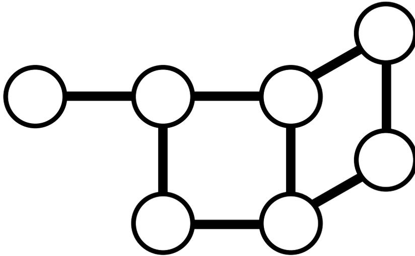
You can ask: “Which nodes (observation towers) do you have to choose at least such that every edge (forest path) is next to a chosen node (observation tower)?” This question is also known as *minimal vertex cover*. It can, for example, be applied when putting up street lights, which should illuminate all streets. Another example is placing cameras, which should cover all hallways.
