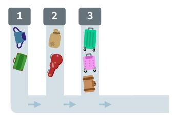
The operators at the check-in counters will place bags one at a time on the vertical lane. As each new bag is placed, the operator presses a button to move the bag forward. When the bag reaches the horizontal lane it will transfer automatically to that lane.
